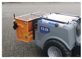
The spreader can hold 100 liters of spreading material but can be quickly increased to 170 liters by mounting a expansion ring.
