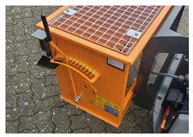
The dosage of the spreading material is adjusted easily and simply with a handle located on the left side of the spreader.
