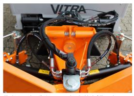
The horizontal oscillation ensures that the blade follows the ground on smaller slopes and in changing terrain
