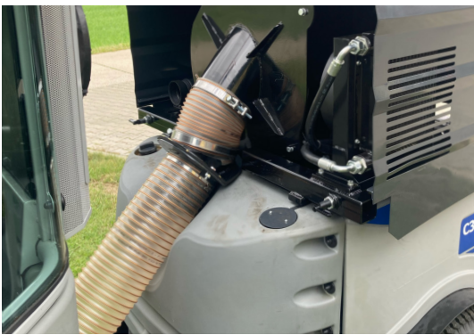
190 mm diameter suction hose for efficient collection.
