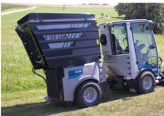
Container volume of 1.2 m 3 and high tip with unloading in 190 cm. and a powerful turbine with high suction power.
