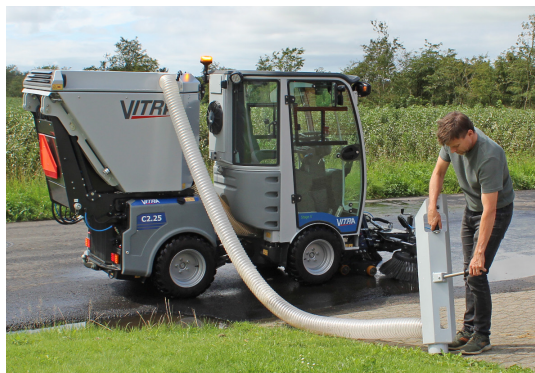
The suction unit is by default equipped with a 6 meter handheld suction hose which ensures great flexibility.
