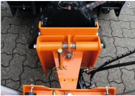
The blade is adjusted to fit Vitra and built with flap inserts to protect the snow balde from direct impact.
