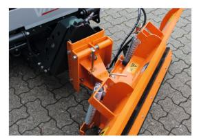
Hydraulic swing directly from the cabin, ensures optimal angle in proportion to the working conditions.
