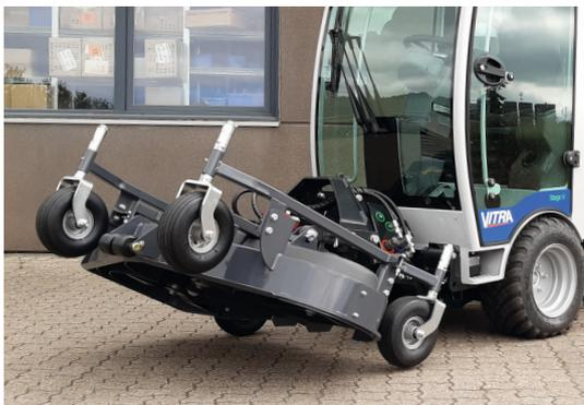
The cutting table can be tilt up for easy cleaning and maintenance. As an option, the mowers can be supplied with hydraulic tilting.
