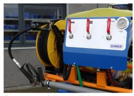
The system is equipped with an external high-pressure cleaner, with hand lance and a 10 meter hose.
