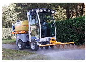
The 1.3 meter wide high-pressure boom is equipped with hydraulic angel adjustment and 8 high-pressure nozzles.
