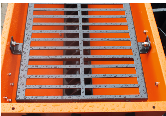
The spreader is equipped with a hydraulic stirrer, which ensures an even spreading of the material.
