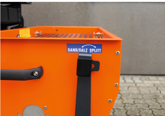
The spreaders can be used with both sand and salt and the switch is made directly on the side of the spreader.
