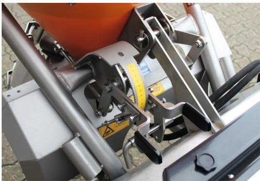
The dosage amount is easily and simply adjusted using a handle that is easily accessible on the spreader.
