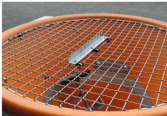
The spreader is equipped with a hydraulic agitator, which ensures an even distribution and uniform spreading.
