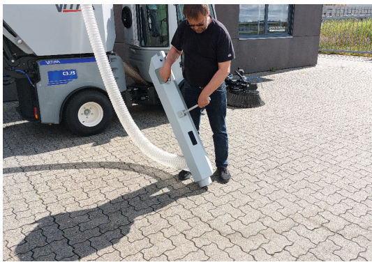
The suction unit is by default equipped with a 5 meter handheld suction hose which ensures great flexibility.
