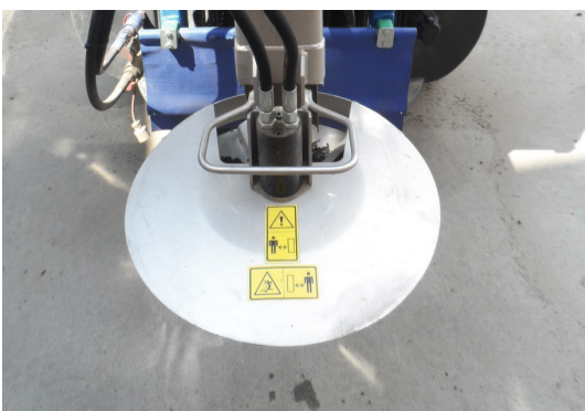
The spreader can be adjusted from 1 to 6 metres spreading width, and can be used for sand, salt and grit.
