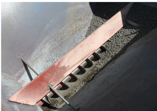
The spreader is fitted with a bottom-mounted auger, which ensures efficient feeding of the spreading material.
