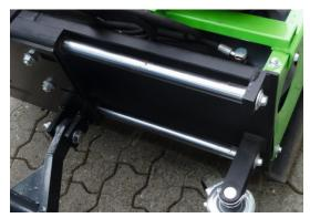
As an option, the system can be delivered with a hydraulic lateral shift, with the option to shift the unit sideways 180 mm. to each side.
