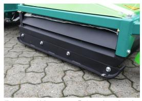
The innovative side burners ensure effective weed control very close to, for example, house walls and curbs, without the risk of collision.
