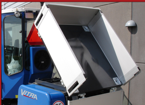
As an option, the truck bed can be mounted with hydraulic tilt for easy unloading.
