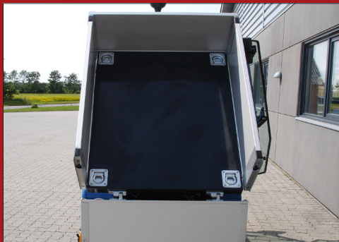
The truck bed is equipped with flat floor, which is equipped with safety hooks in each corner.
