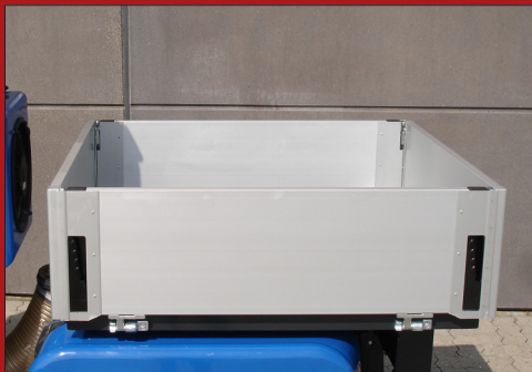
The truck bed is built as a strong steel/aluminium construction, which ensures low weight and large load capacity.
