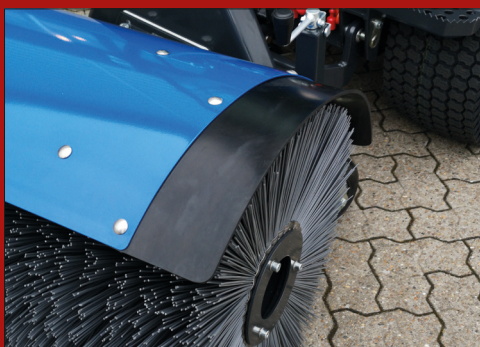
The brush guard is equipped with rubber edges that protect against damage in the event of a collision.
