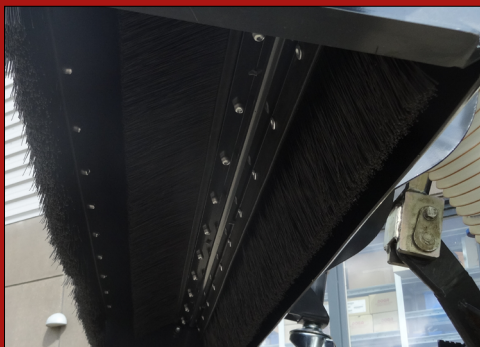
The suction head effectively collects leaves from the pitch without removing granulate from the bottom of the field.
