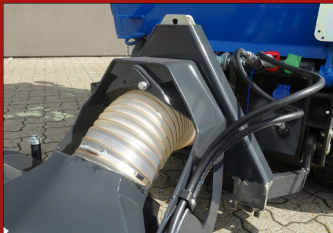
The front is built with a standard A-frame – Cat. A and can therefore be installed on a variety of machines.
