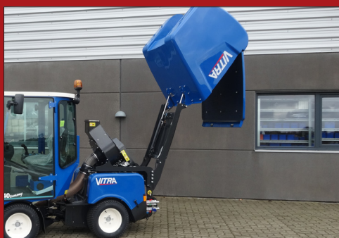
The collector has unloading height of up to 190 cm, to ensure a lot of tipping possibilities for the driver.
