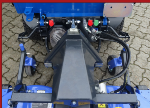
The mowing deck is mounted with a standard A-frame and equipped with strong stabilisers
