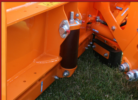
The suspended flap is divided into three sections, so only the part that hits an obstacle folds backwards.
