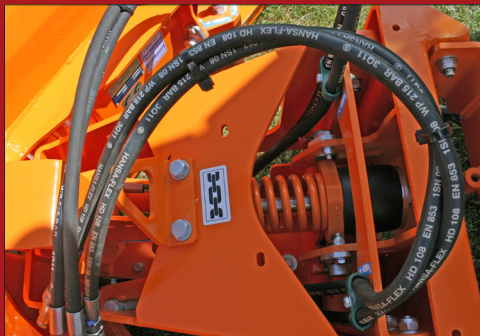
The V-Plough is built with a horizontal flex-suspension system, to protect against direct impact
