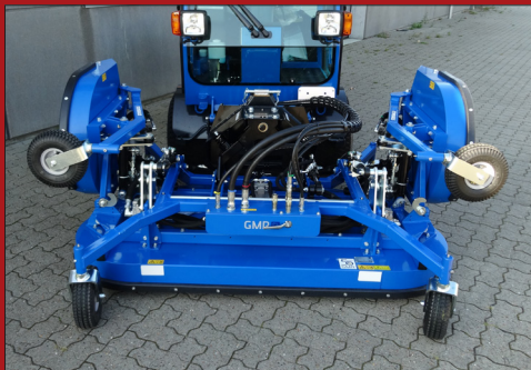
The hydraulic side-wings make it possible to easily transport the mower through traffic, despite its large working-surface.
