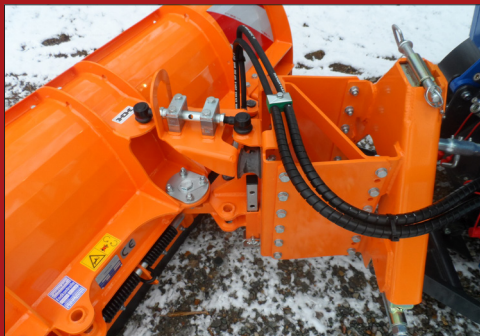
The blade is by default mounted with hydraulic adjustment of the working angle.
