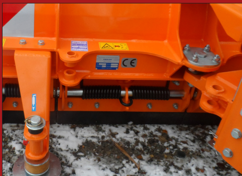
The flap inserts that are divided ensure that the blade is folded backwards in case of impact.
