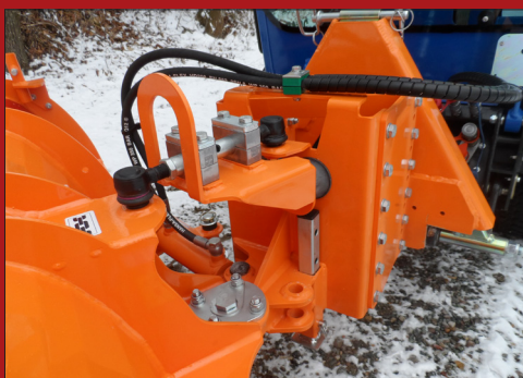
The blade is mounted to a suspended mounting which is built on a standard A-frame.
