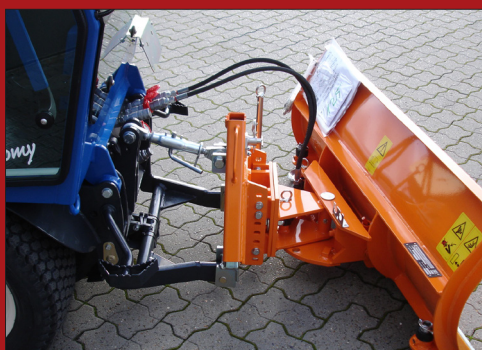
The blade is adjusted to fit Vitra and built with flap inserts to protect from impact.
