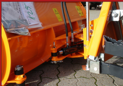
Hydraulic swing ensures optimal angle in proportion to the working conditions.
