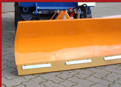
The strong synthetic list ensures a good compromise between performance, noise and durability.
