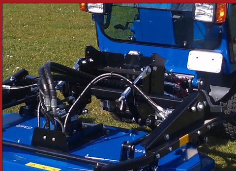
Additionally the cutting height can be hydraulically adjusted, which can easily be done by the driver directly from the cabin.
