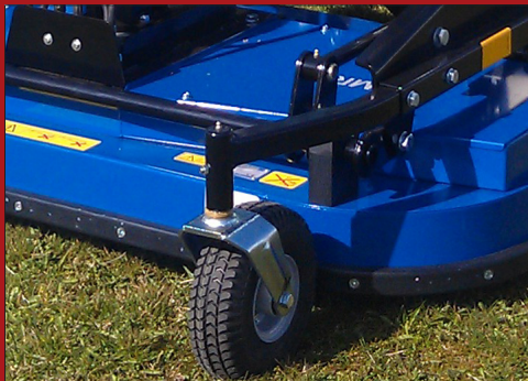
The mower is installed with strong rubber-support wheels in the front and back to ensure optimal stability.
