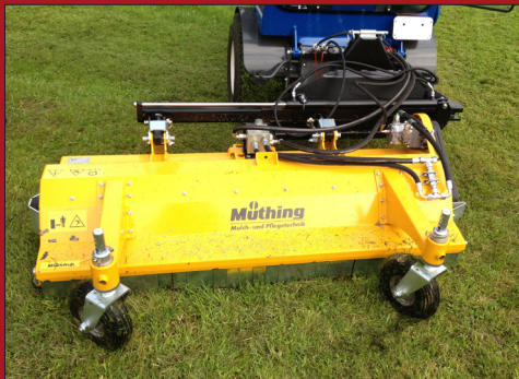
As an option, the mower can be shipped with hydraulic side-shifting, which gives even more flexibility.
