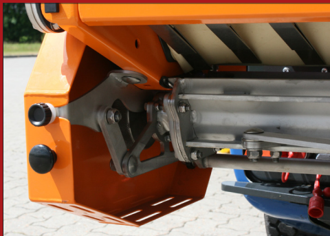
Switch between roller- and disc spreader and spreading width adjustment is done easily and comfortably from the cabin.
