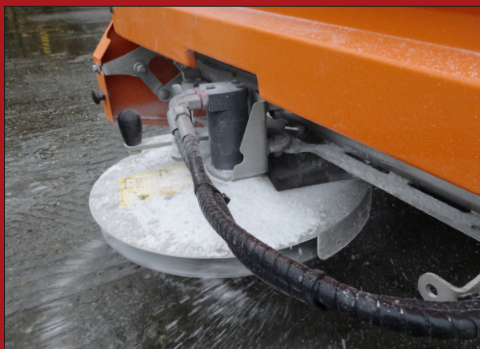
All parts of the spreader are made from either stainless steel or lacquered with varnish in corrosion-class C5.
