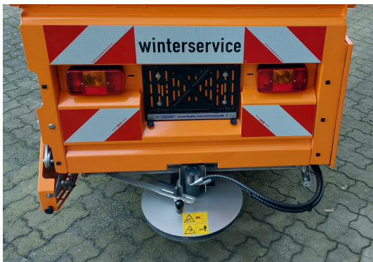
All components are made of stainless steel or are coated in the C5 corrosion class, ensuring a long service life for the spreader.
