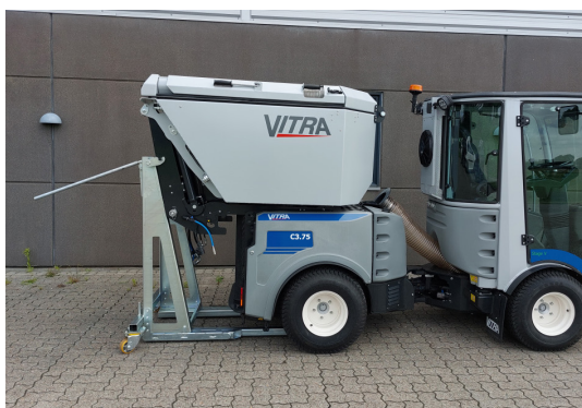
Despite the high capacity, the container can be easily and fast mounted on the machine with the Vitra Quick-Shift system.
