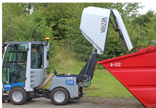
The container is emptied without leaving the cabin and takes place at 175 cm. height, so emptying can take place directly in containers.
