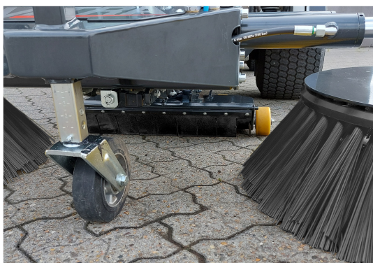
The wide suction head is equipped with a hydraulic flap which ensures easy collection of larger pieces of waste.
