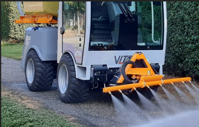
The wide selection of attachments also includes a washing system with a flush boom and the option of a high-pressure cleaner
