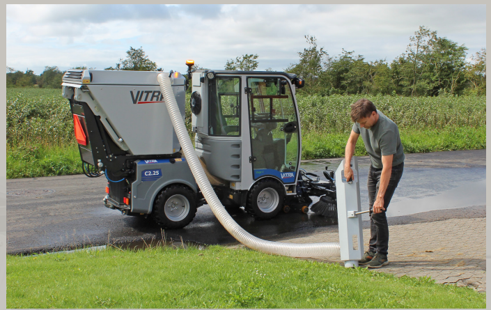
With the external suction hose, there is the possibility of efficient cleaning where it is not possible to drive the machine
