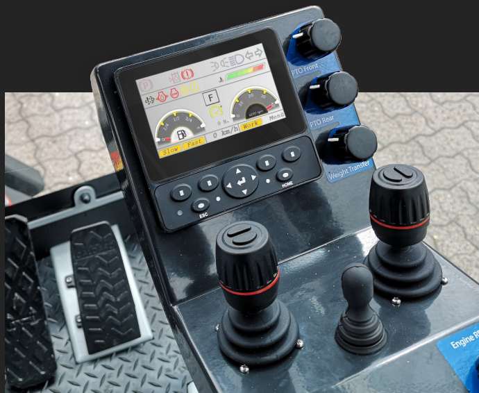
The C3 Series is easily maneuvered with the 2 proportional joysticks, which ensure that the intuitive operation can be performed precisely
