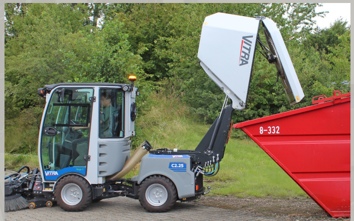
The container is emptied from the cabin and with a unload height of 175 cm. emptying can take place directly in a container or trailer
